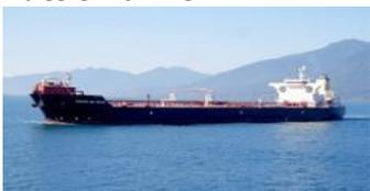
Tankers that transport crude oil from offshore oil rigs, such as FPSOs, to onshore refineries as an alternative for pipelines. Shuttle tankers are fitted with a unique system that enables cargo to be loaded from the bow of the vessel, rather than from the side like ordinary tankers, while maintaining a certain distance from the offshore platform.
