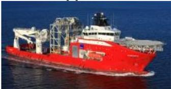
A working vessel for the installation, maintenance, and recovery of seabed facilities necessary for the development and production of offshore oil and gas fields.
