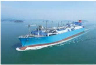
An LNG vessel that is equipped with the facility for storing and regasification of LNG, which is then pressurized and piped ashore. Plans to introduce FSRUs in regions around the world are making steady progress as they can set up LNG receiving terminals in shorter amount of time and with less cost than conventional onshore receiving terminals.
