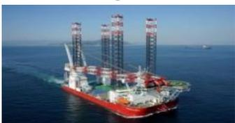
A vessel equipped with legs that rest on the seabed and a platform that moves up and down. The vessel installs offshore wind power generation systems with a crane by moving the platform up to the sea surface. In addition to installing offshore wind power generation systems, it can engage in supporting maintenance of offshore oil and gas rigs.
