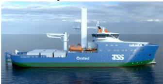
SOV has accommodation for maintenance technicians working on wind turbines that makes a offshore wind farm, allowing them to stay on-site for extended periods. SOV constantly maintains a safe distance from the offshore wind farm (= Dynamic Position System), and equipped with motion compensation function gangway. This allows technicians to move safely between the vessel and the offshore wind farm.
