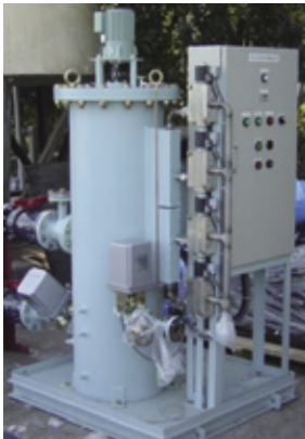
Ballast water disposal system
