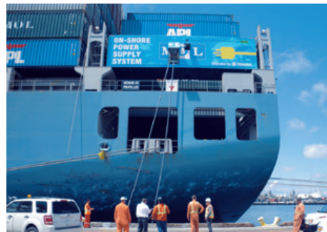
The containership MOL Matrix using an onshore power supply system
