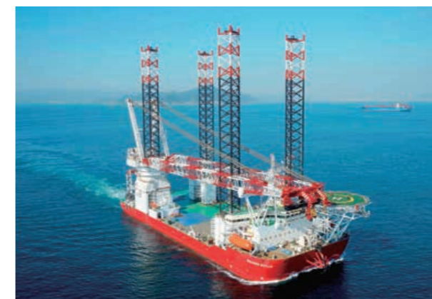
One of the world’s largest Self-Elevating Platform vessels, the Seajacks Scylla, owned and operated by Seajacks
