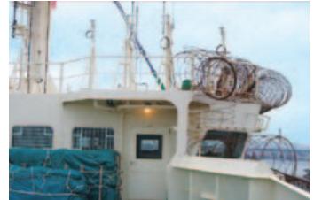
Razor wire is installed around the periphery of the bridge
