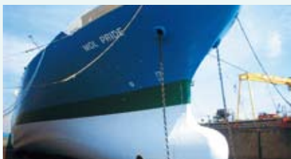
A Containership Coated With Silicon Resin Paint (MOL Pride)
