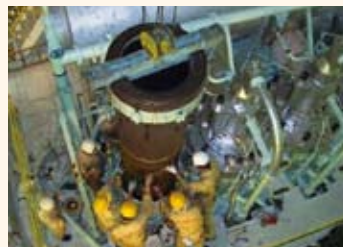
Engine Department: Removing a piston from the main engine
