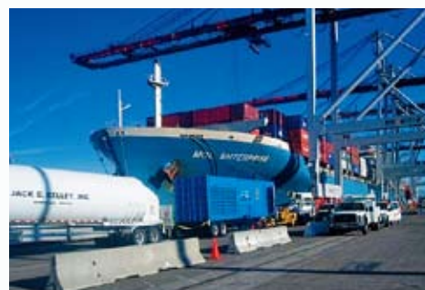
The MOL Enterprise receives power from an on-shore generator.
