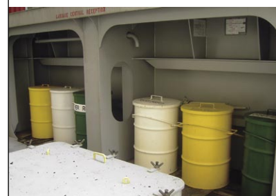
Vessel trash separation and collection site
