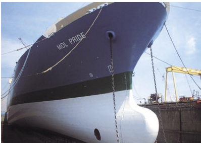
Containership coated with silicon resin paint
