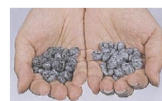
Commercial recycling of aluminum pellets (right) and steel pellets
