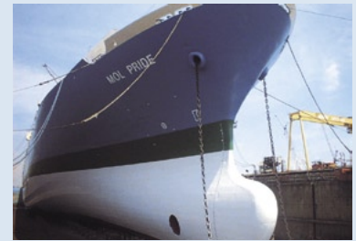
Containership coated with silicon resin paint
