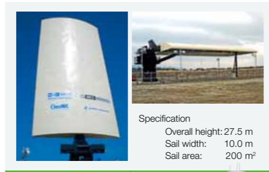
Power Assist Sail prototype
