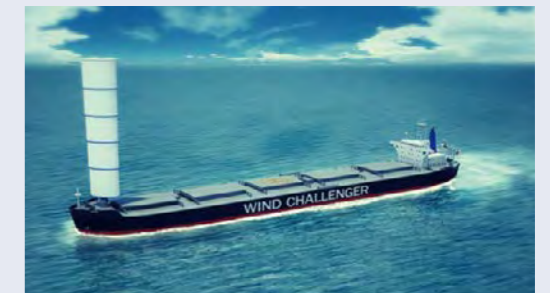
Conceptual image of the vessel equipped with a single sail while in full sail at sea
